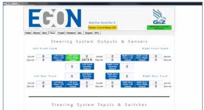
EGON IntelliMatics™ is a powerful remote diagnostics/monitoring system. The G&Z software engineering team has designed a web based remote user interface to allow maximum connectivity anywhere in the world for the contractor as well as for solving challenges with G&Z service personnel.
