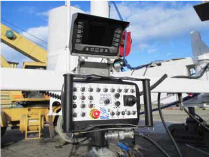
EGON Belly Pack console provides great flexibility to the operator. With the option to mount the entire console with the LCD display on any sensor arm or take the console remote, the EGON Belly
