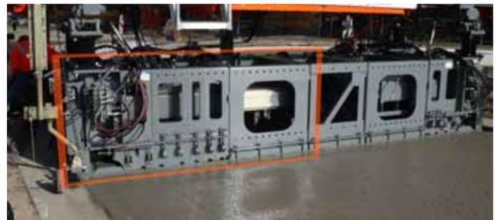
The TeleEnd: Telescopic Paving Kit End Section offers 3 ft (1m) of quick change kit per side. A 6 ft (2m) width change can be accomplished by one or two people in as little as an hour. Larger TeleEnds available up to 6.5 ft (2m) per side.
