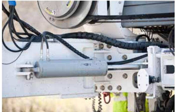
The SmartLeg system allows contractors to adjust the swing leg angle on-the-fly to maneuver around an obstacle without stopping production.
